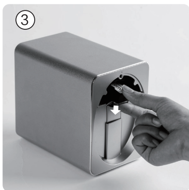
3. Hold the front part of the cartridge, press down and take it out.
